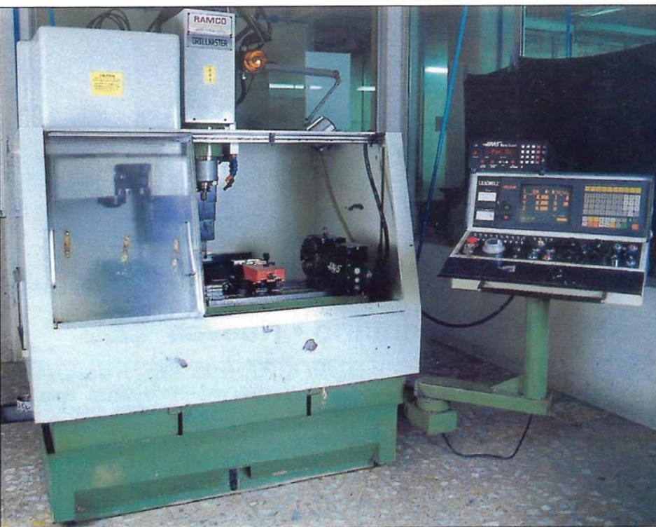
CENTROS DE MAQUINADO CNC VERTICAL, MARCA: LEADWELL LEADWELL CNC VERTICAL MACHINING CENTER
